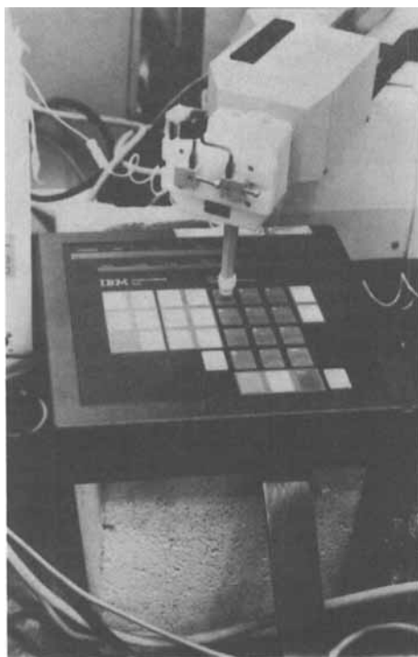
Figure 27. The Zymate robot programs the keypad of an IBM-LC9533 ternary gradient liquid chromatograph. This illustrates the principle of a "soft" instrument interface.
