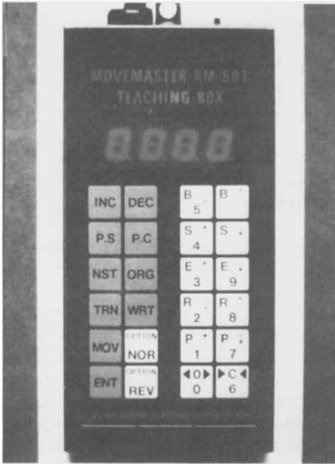
Figure 16. The teaching pendant for the P.E. Masterlab robot.
