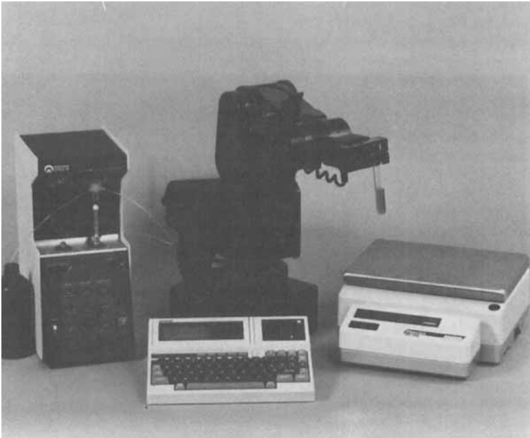
Figure 5. The JOSCO-SMARTARM™ robot shown with an Epson HX-40 computer, a digital balance and a digital pipet.
