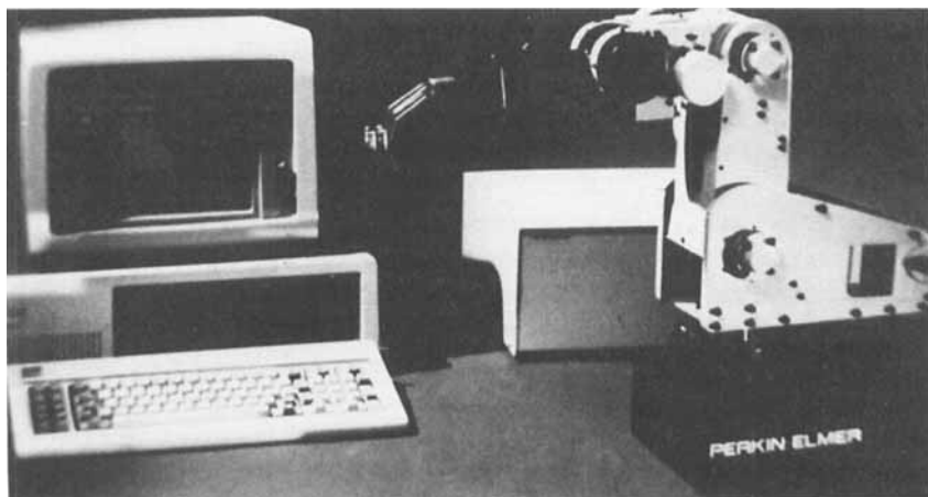
Figure 14. Photograph of the P.E. Masterlab robot shown with its controller, an IBM-PC.
